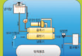
빙축열시스템 (Ice Storage System)
